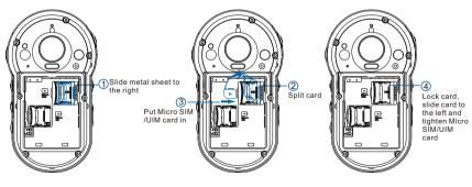
After pulling out the battery, insert Micro SIM/UIM card and TF card into the device. [Notice] Some models do not support SIM card slot. The method of installing a TF card is the same as that to install a Micro SIM/UIM card.
